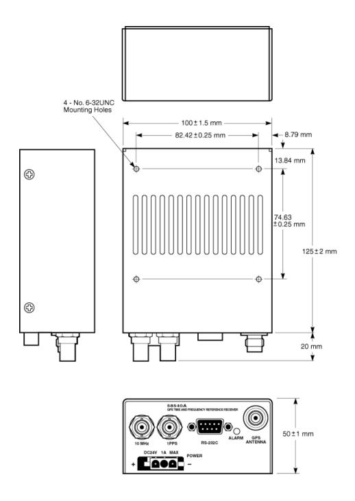
Figure 3-2. 58540A External Diagram (Standard Configuration)
