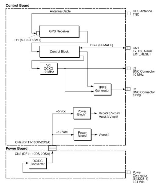
Figure 3-1. 58540A Functional Block Diagram
